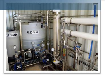
Basic container pilot plant utilizes 4" membranes to achieve a higher permeate production rate for downstream evaluation:
